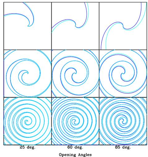
FIG. 5.— This plot shows different opening half-angles  $\beta$  of the cavity/compression and then zooms out to reveal a top view of the projected spiral path in the orbit plane. The eccentricity of the orbit is fixed at 0.5.
